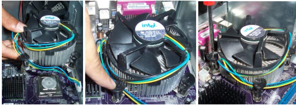
Gambar 3. 7. Memasang Heatsink Prosesor
