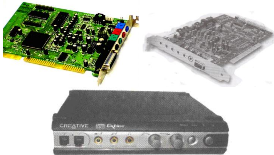
Gambar 2. 21.Sound Card Model ISA, PCI dan Sound External
